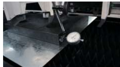
04 VERTICALITY INSPECTION Checking the perpendicularity of the marble inspection bed.
